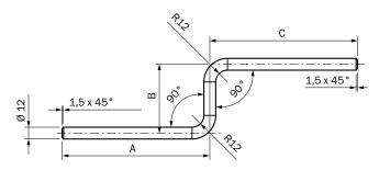
A = 150 mm, B = 70 mm, C = 150 mm (BEF-MS12Z-A) A = 150 mm, B = 70 mm, C = 250 mm (BEF-MS12Z-B)
