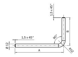
A = 150 mm, B = 150 mm (BEF-MS12L-A) A = 250 mm, B = 250 mm (BEF-MS12L-B)
