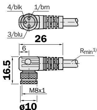
**Female connector M8, 3-pin, PUR halogen-free, straight**
