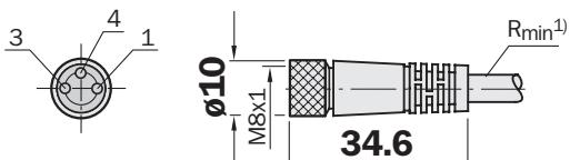
**Female connector M8, 3-pin, PUR halogen-free, angled**
